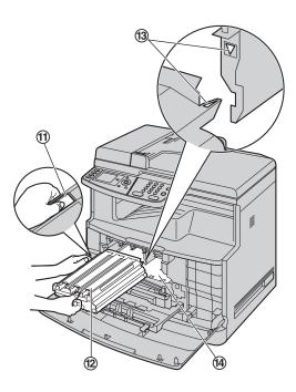
9 Remove the monochrome drum cartridge from the protection bag.
